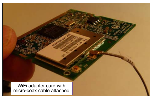
Figure 4 Cable attached and adapter card ready to install.
