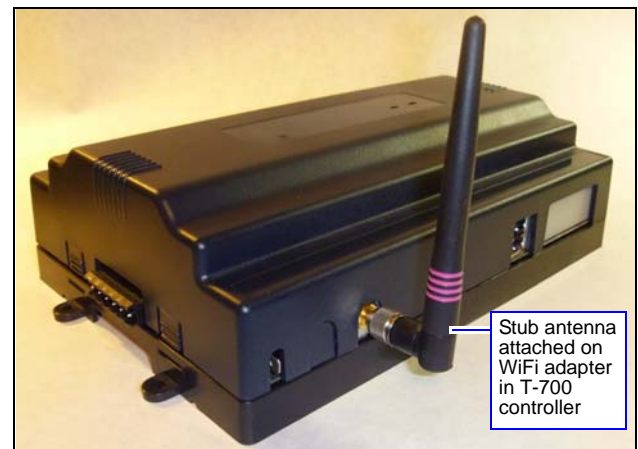
Figure 22 RP-SMA stub antenna on controller.
